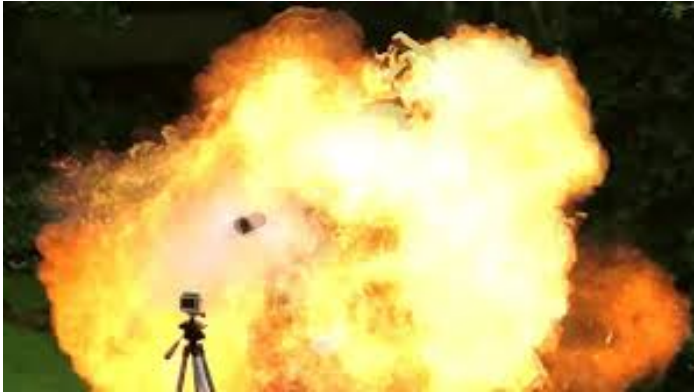
(Examples of an exploding aerosol can under BLEVE conditions)
