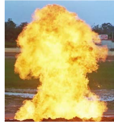
(Examples of an exploding aerosol can under BLEVE conditions)
