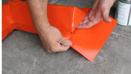
5. Press together when tacky and fold excess PVC under the foam.
